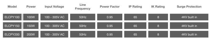
Protection: Over current - Constant current limiting, recovers automatically after fault condition is removed. Short circuit - Hiccup mode, recovers automatically after fault condition is removed. Over Voltage - Shut down and latch off o/p voltage, re-power on to recover. Meanwell HLG Driver. Vibration: 10 ~ 500Hz, 5G 12min./1cycle, period for 72min. each along X, Y, Z axes
